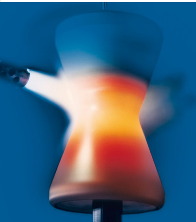
Automatic fusing of CrNi BoSi alloy sprayed on rope pulley by means of the powder flame-spraying process.
